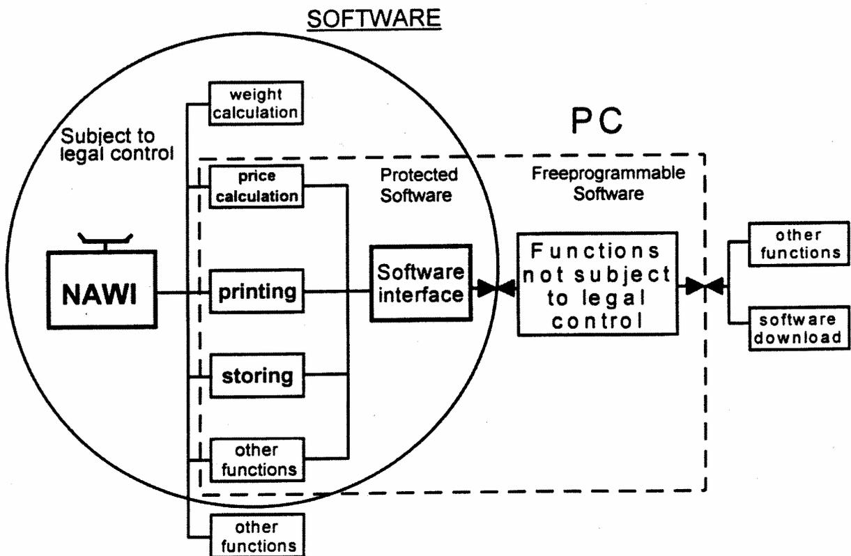
**Figure 2:** Example of a software structure of a PC-based weighing system
